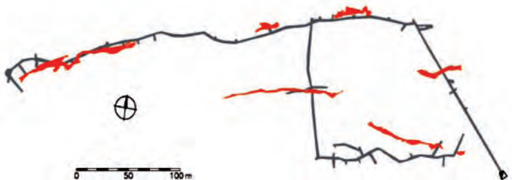
Remaining mine galleries (grey) and natural caves (orange) that have been intersected during mining
